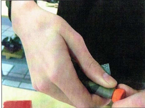
First of all I had to sand al of the little parts I used, as they were 3D printed they had lots of imperfections.
