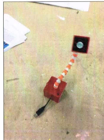
These imperfections had to be sanded away as they needed to fit one another and also to be smooth to increase it's ergonomics.
