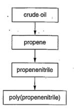
(a) Long chain alkanes such as  $C_{17}H_{36}$  can be cracked to form propene,  $C_3H_6$ .
