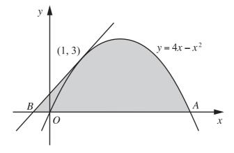
The diagram shows the curve  $y = 4x - x^2$ , which crosses the x-axis at the origin O and the point A. The tangent to the curve at the point (1, 3) crosses the x-axis at the point B.
