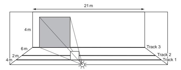
The screen is 21 metres wide and 4 metres high, and the light source is 12 metres behind the screen, in the centre at floor level. The lighting director is able to place her squares on any of three tracks running parallel to the screen. Track 1 is 8 metres from the screen, track 2 is 6 metres from the screen and track 3 lies right next to the screen.
