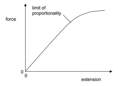
The work that must be done to extend a spring is equal to the area under the force-extension graph.
