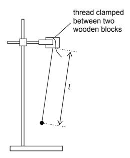
2 Practice a few times releasing the pendulum and timing ten complete swings. A complete swing is when the pendulum bob moves:
