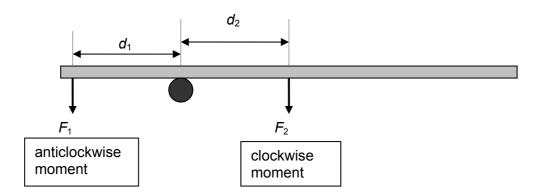
If the rule is balanced, we can apply the principle of moments. This results in the equation
