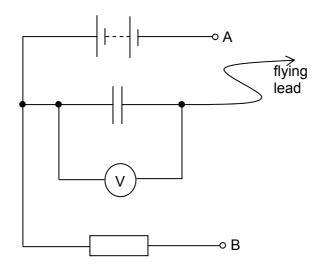
When a capacitor of capacitance C is discharged through a resistor of resistance R, the potential difference  $V_t$  across the capacitor at time t is given by the equation.
