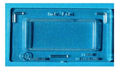
Figure 8.1 A Sedgewick-Rafter counting chamber [Photo © John Adds]
