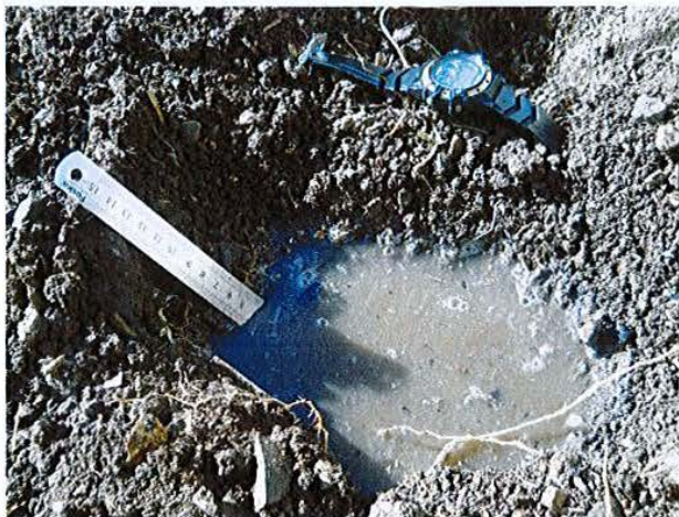
Figure 2: Step 2 of percolation test
