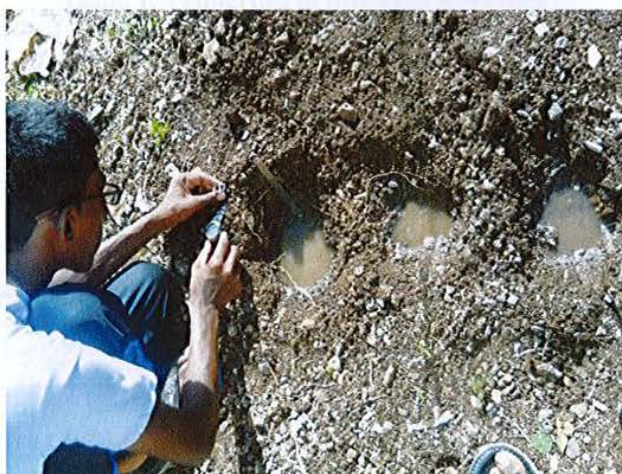
Figure 2.1: Step 3 of percolation test
