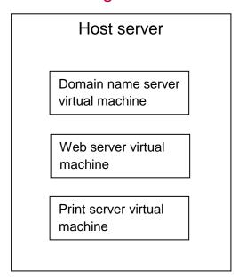
If a host system is powerful enough, several virtual machines can be run side-by-side on one computer. A good example of this is the increasing use of virtual machines to run several virtual servers, such as a domain name server, web server and print server, on one physical server. The host server maintains the virtual machines and allows them to act as though they are all separate computers.
